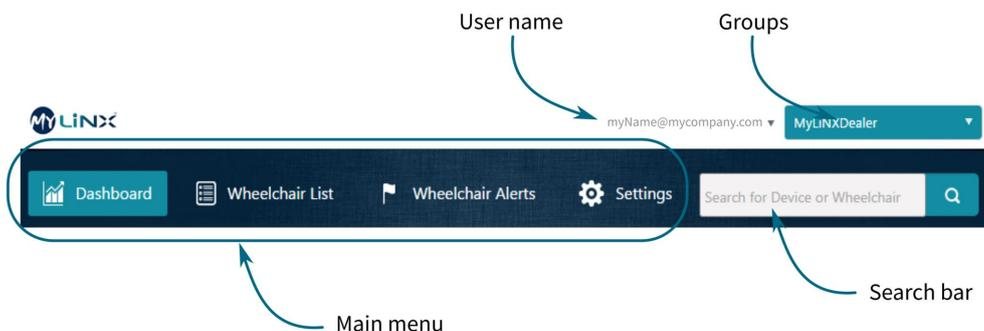
Figure 4: MyLiNX common control panel
