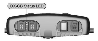
A flashing DX-GB-AS Status LED indicates there is an abnormal condition somewhere on the powerchair. The components that DX provides fault information for include, the motors, the park brakes, the batteries, the cabling and the DX modules themselves. The Flash Code displayed on the DX-GB-AS may be different to that displayed by the DX System Status LED located on the DX Master Remote.
