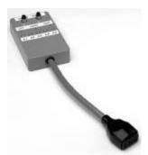
With the wheelchair turned off, disconnect the 21 way lighting/actuator connector, and replace with the DX CLAM tester. Turn the wheelchair back on, operate all functions via the remote as normal. Check to ensure all functions operate correctly.
