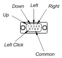
**Figure 7** – Typical ECU Mouse Mover Connections
