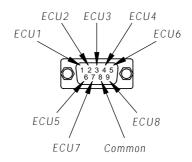
Figure 6 – ECU DB9 Connections
