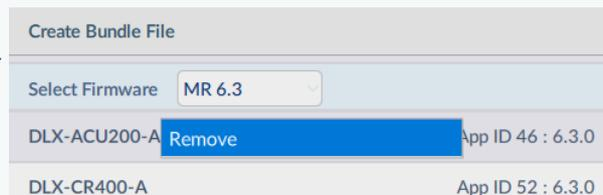
Figure 135: Removing firmware files
