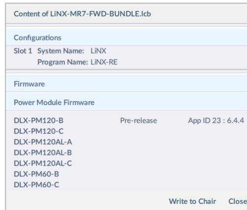
Figure 140: Writing the bundle file to the connected system
