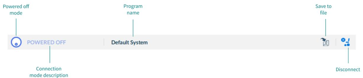
Figure 31: Toolbar - connection context - powered off
