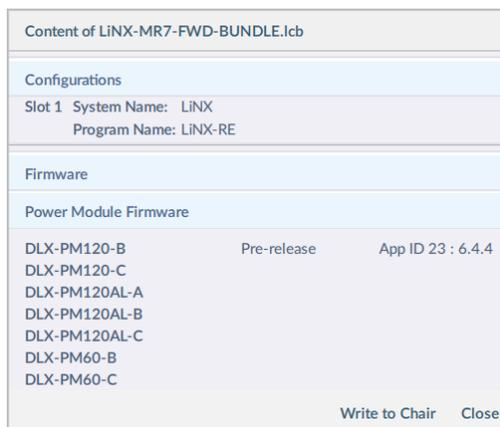
Figure 142: Writing the bundle file to the connected system
