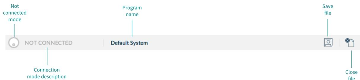
Figure 32: Toolbar - connection context - no connection
