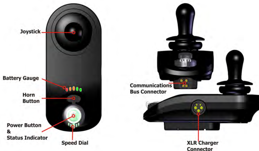
Figure 36: The Remote REM050: user interface and connectors
