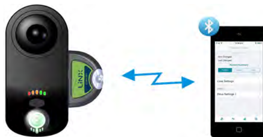
Figure 54: Programming and diagnostics with the LiNX Access iOS tool
