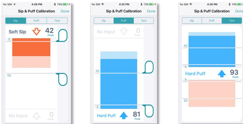
Figure 41: Sip and Puff calibration and test screens
