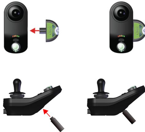
**Figure 4: Inserting the LiNX Access Key**
