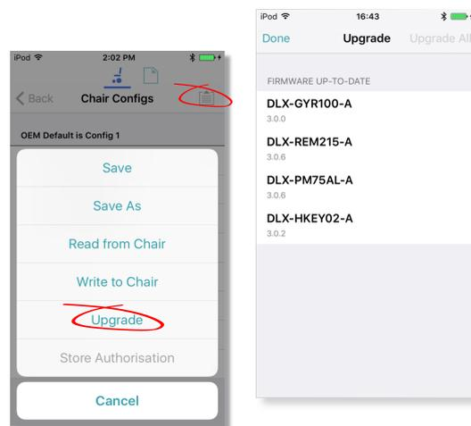
Figure 37: Upgrading the firmware
