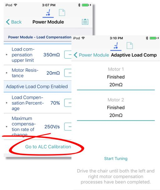
Figure 39: Tuning Adaptive Load Compensation
