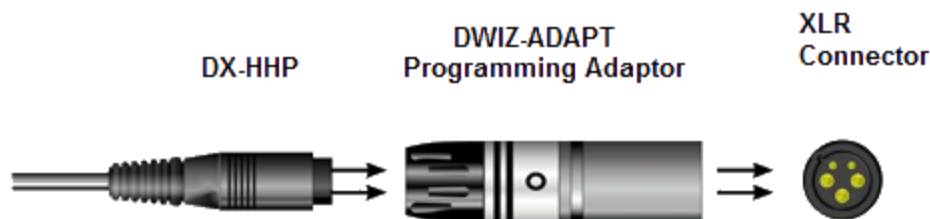
Figure 72: Connecting the DX-HHP
