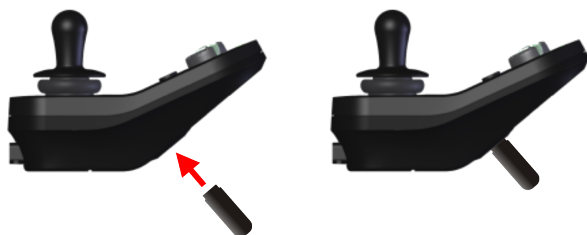
Figure 33: Inserting the LiNX Access Key into the REM060
