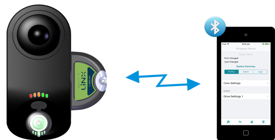
Figure 29: Programming and diagnostics with the LiNX Access iOS tool
