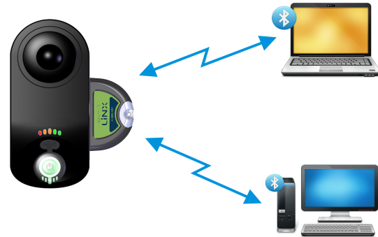
Figure 30: Programming and diagnostics with the LiNX Access PCtool using a LiNX Access Key
